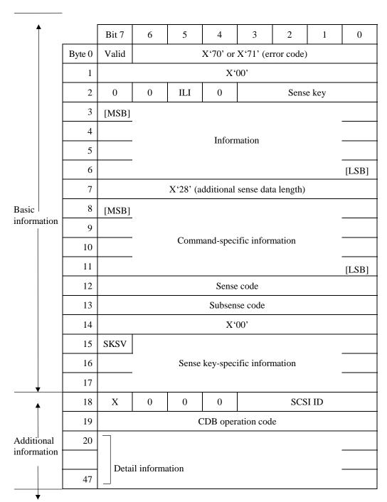
Figure 7.1 Format of extended sense data
